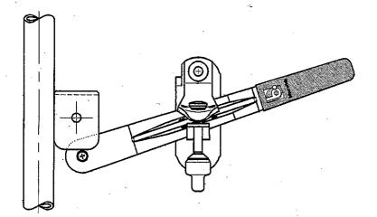
The long reach handle hub with a 3 - point catch and retainer prevents disengagement of handle in the event of rivet removal.
