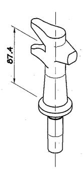
Still incorporating the robust long bodied design. The wider cam shoulder improves the resistance to racking loads.
