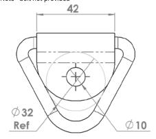
Model No. BCP16010 (Mild Steel) Model No. BCSP16010 (Stainless Steel)
