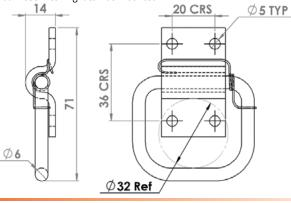
Model No. BCP16011 (Mild Steel) Model No. BCSP16011 (Stainless Steel)
