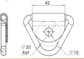
Model No BCP16010 (Mild Steel) Model No BCSP16010 (Stainless Steel)
